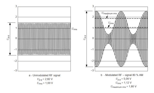
Consequently, the level of the modulated signal must be 5.1 dB higher than the test levels specified by the standard. The insertion loss of a typical CDN is approximately 10 dB from RF input to the output of a 150 Ohm to 50 Ohm adapter at the EUT port. Adding a 6dB attenuator to improve matching of the RF power amplifiers would require following amplifier output power:
