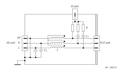
CDN-M3,  $C_1$  (typical) = 10 nF,  $C_2$  (typical) = 47 nF,  $R = 300 \ \Omega$ ,  $L \ge 280 \ \mu\text{H}$  at 150 kHz CDN-M2,  $C_1$  (typical) = 10 nF,  $C_2$  (typical) = 47 nF,  $R = 200 \ \Omega$ ,  $L \ge 280 \ \mu\text{H}$  at 150 kHz CDN-M1,  $C_1$  (typical) = 22 nF,  $C_2$  (typical) = 47 nF,  $R = 100 \ \Omega$ ,  $L \ge 280 \ \mu\text{H}$  at 150 kHz
