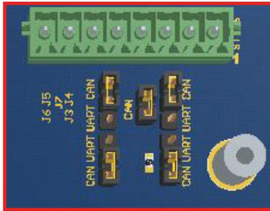
Abb. 6: Jumper CAN/UART/I2C
